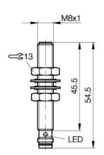
**Inductive Sensors** BES 516-324-S 49-C M8x1 x 54.5 normally-open Sn=1,5mm shielded
